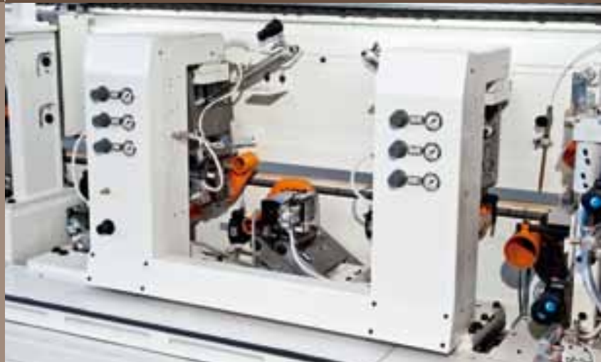
Multifunctional 4 motors corner rounding unit
