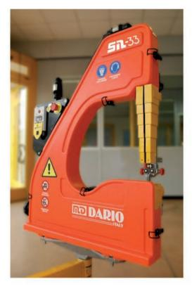
The main feature that distinguishes MD DARIO bandsaws from conventional models is the ARTICULATED ARM, that with a special system of joints, allows the machine to rotate in every direction so that the user can perform creative and precise cuts.
