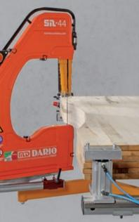
This device involves a special PNEUMATIC MATERIAL SUPPORT with pneumatic hold-down device.
